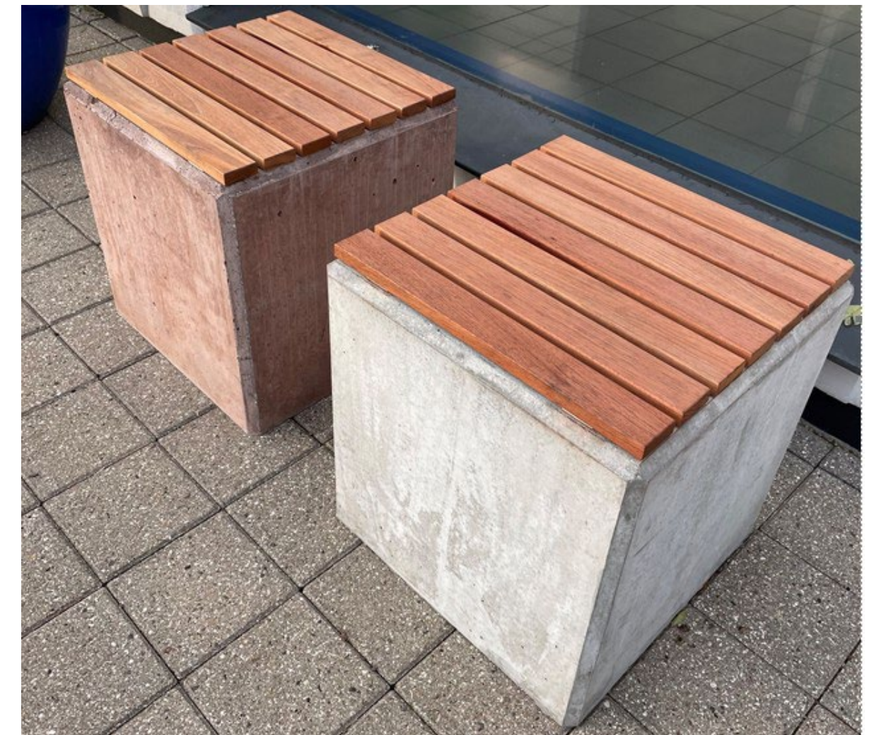
Test benches made by a cement / leaching residue blend with and without the Sahara module (source: EasyMining)
