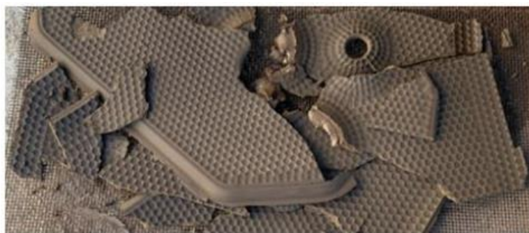
Figure 4. Press cake obtained with the membrane filter press during the long duration experiment.
