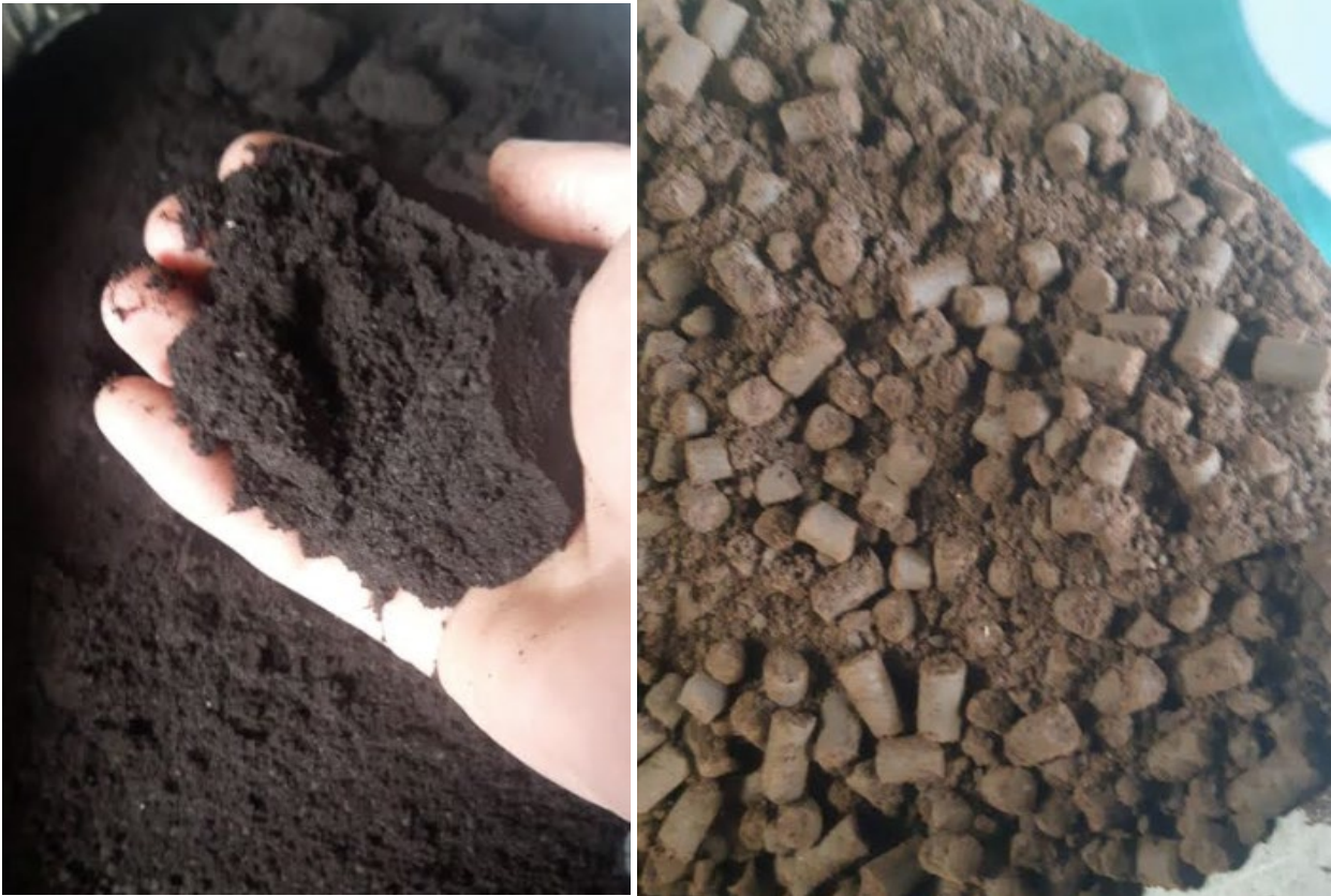
Figure 9: Olive Pellets – soft and powdery
