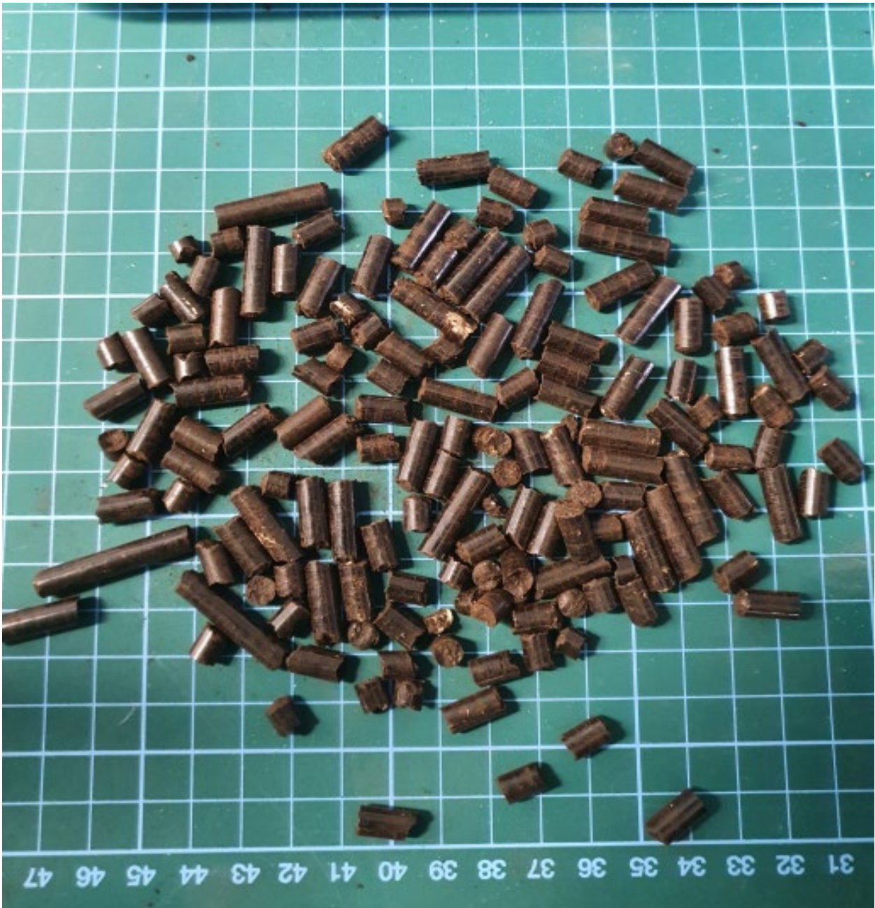
Figure 7: Orange Pellets – mechanically strong and easy to handle
