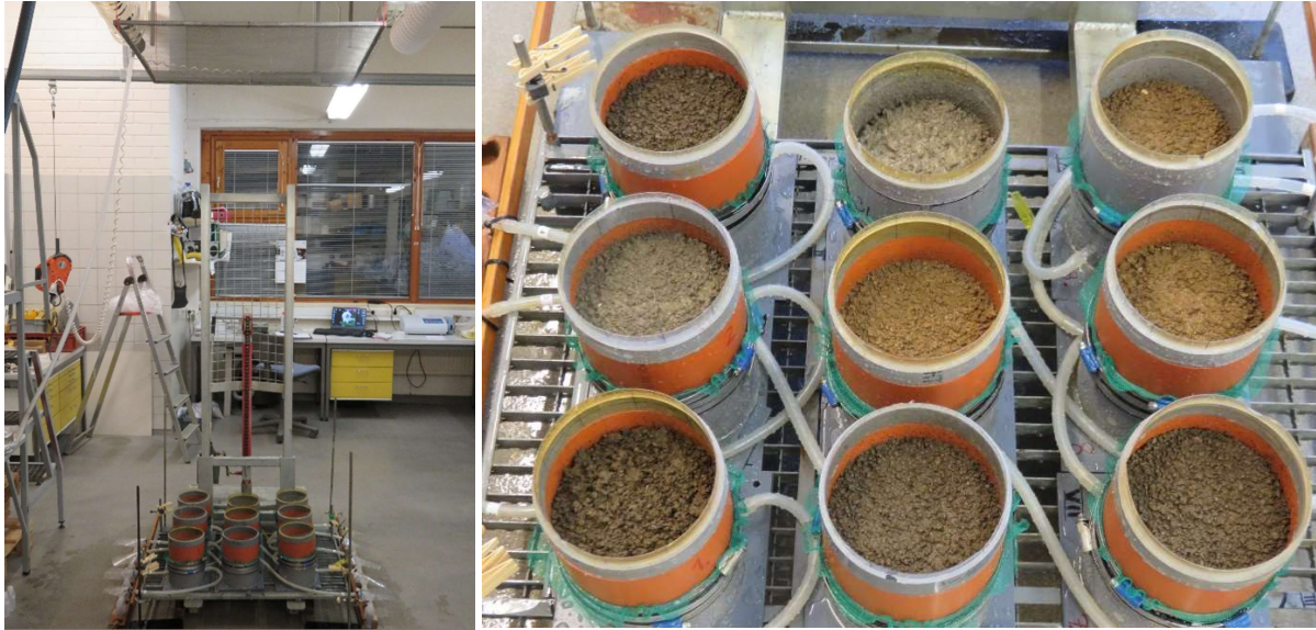
Figure 8. Rainfall simulation for studying nutrient losses after application of BBFs in soils originating from Spain, Germany, and Finland.
