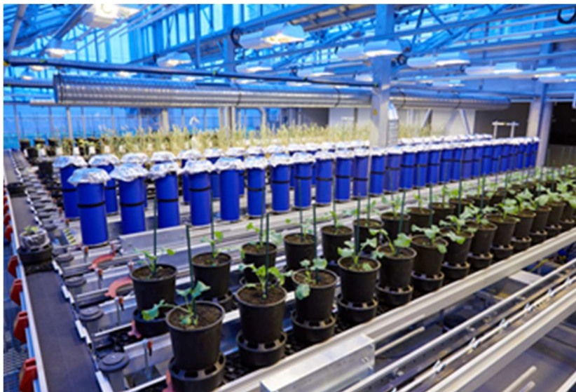
Figure 7. Phenotyping platform for visualizing crop growth, both shoot and root growth, caused by different BBFs.
