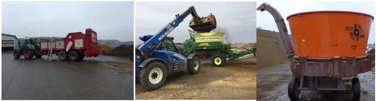
Cutmaster, I-grind och Rotogrind, three options for cutting the unused silage in pieces of optimal size for anaerobic digestion at Jordberga Biogas Plant.
