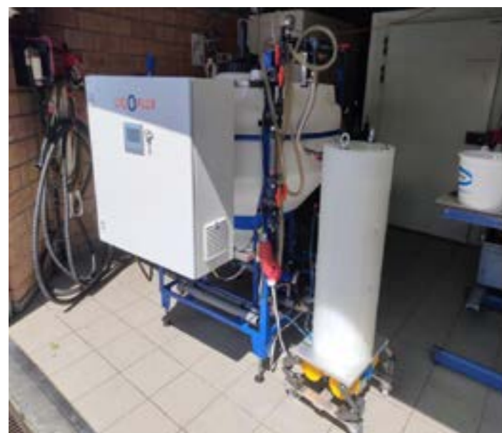
Figure 22: Harvesting (or dewatering) system used at Innolab
