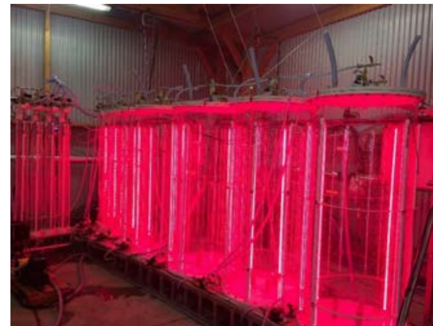
Figure 8 - The photobioreactor with LED lights
