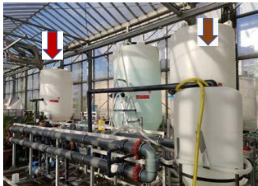
Figure 2: Membrane filtration system showing membrane filtration rig (red arrow) and concentration tank (brown arrow).
