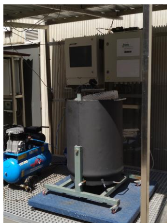
Fig 1: Biodrying pilot unit for the valorization of fish sludge and dead fish
