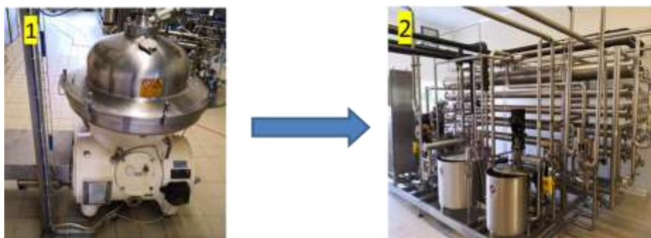
Figure 36: Treatment train for acid whey thickening: (1) centrifuge and (2) nanofiltration unit
