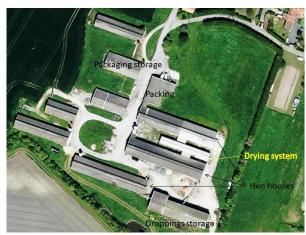
The poultry droppings are collected on treadmills in the hen houses and brought to a drying tunnel. The system uses the heat collected by the ventilation of the air in the hen houses. The transformed poultry droppings are brought with a conveying tunnel in a storage to be mixed and homogenized and to be stocked.
