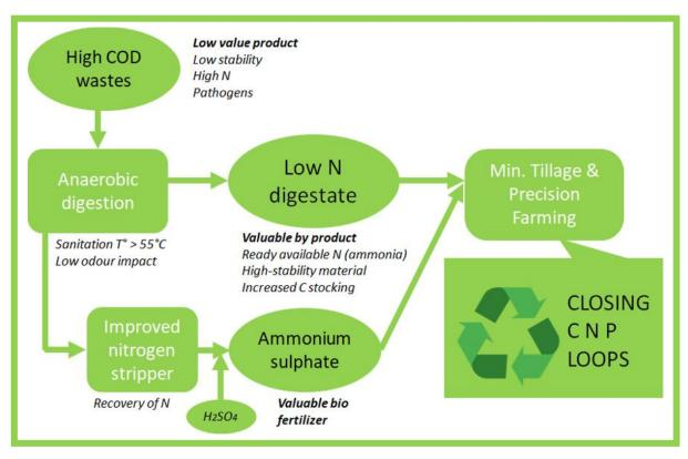
This technique is a complex synergy of technologies to process wastewaters, OFMSW, and agro/food industrial wastes. It includes AD, ammonia stripping system, bio-fertilizer and soils enhancers production, nutrients recycling, precision farming and minimum tillage tools to run effectively rice-culture.
