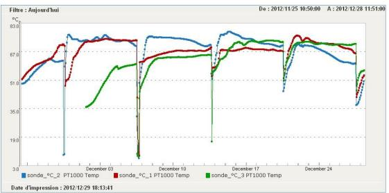
Each coloured curve matches to the temperature monitoring by a different probe on the windrow.
