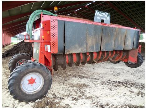
The purpose is to keep the temperature higher than 55°C during five weeks. The moisture is assured with the rabbit liquid manure.
