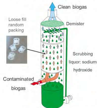
Packed tower scrubber for \text{H}_2\text{S} removal
