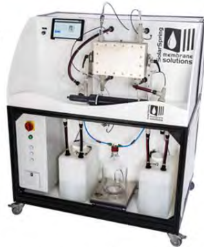
MD bench scale experimental set-up
