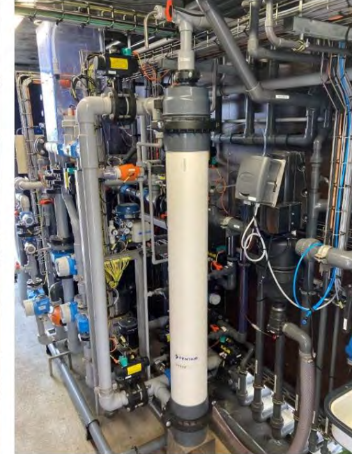
Reverse osmosis membranes Pilot B (novel UF membrane)
