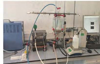
RO bench scale experimental set-up
