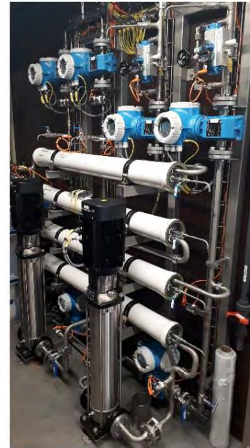
Reverse osmosis membranes Pilot B (novel UF membrane)
