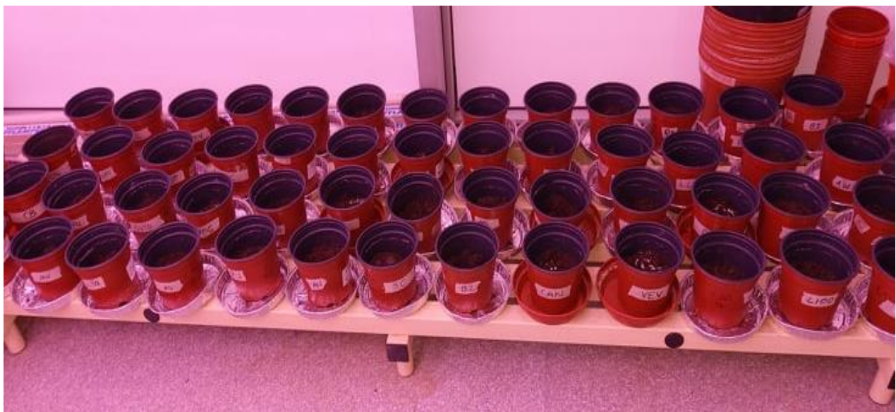
Figure 4. Pot trial setup for testing for the presence of weeds in RDFs.
