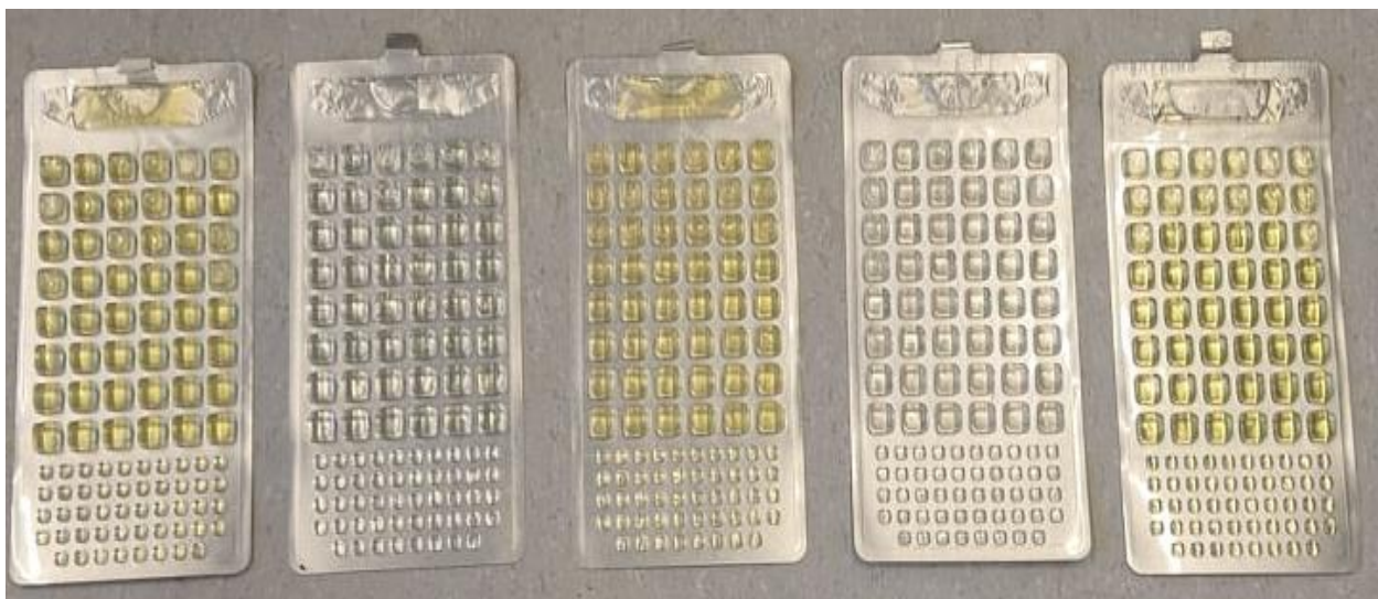
Figure 5. RDF samples in Quanti-Trays after the 18-hour incubation period. From left to right, the samples are blend 1, sterile water, liquid concentrate, struvite from potato processing and pig urine. The faint yellow colour change is visible in blend 1, liquid concentrate and pig urine.
