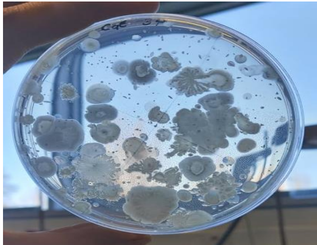
Figure 2. Example of total viable bacteria count (liquid concentrate on plate count agar).
