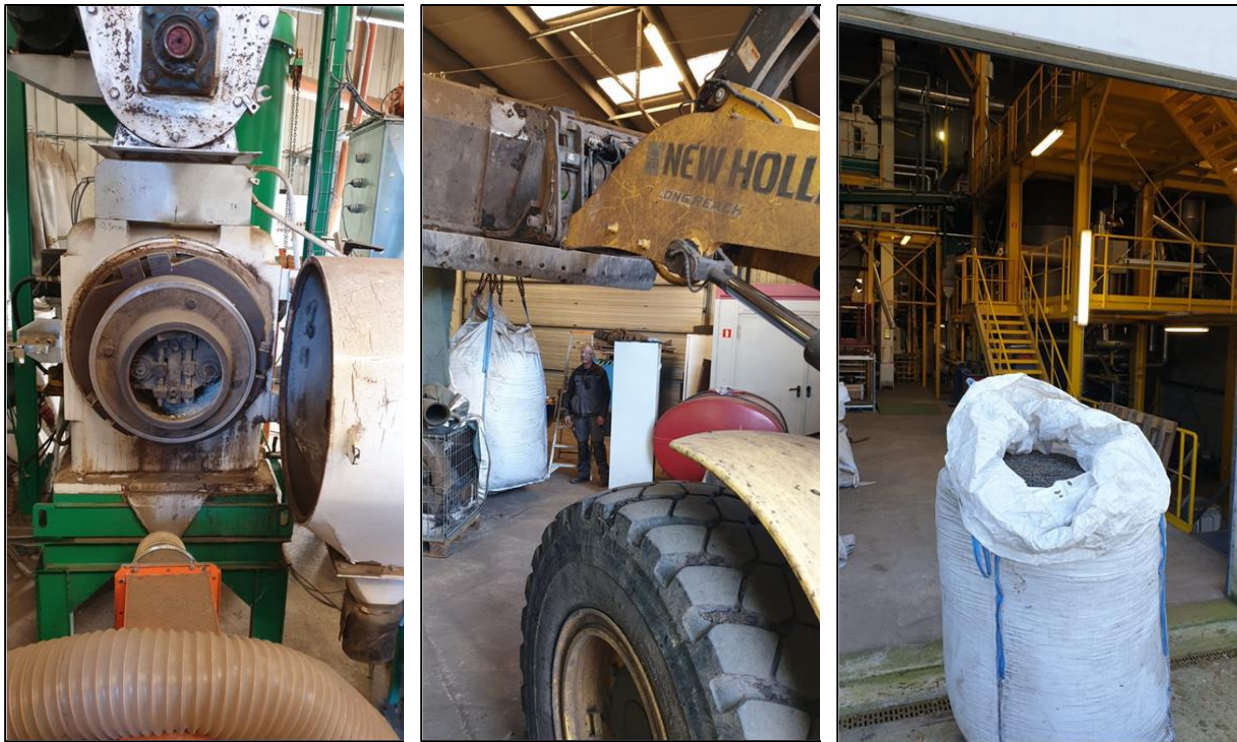
Figure 18. Production of the pellets and preparation for induction into the gasifier
