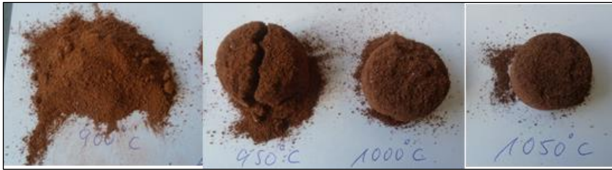
Figure 1. Sample after heat treatment in the muffle furnace at different temperatures
