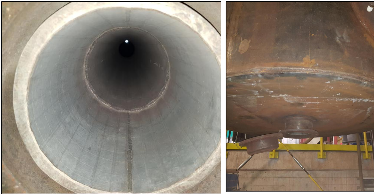
Figure 16. Gasifier interior view (left) and ash discharge (right)
