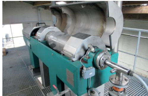
Figure 2-1 Horizontal decanter centrifuge Source: (Gorissen and Snauwaert 2018)
