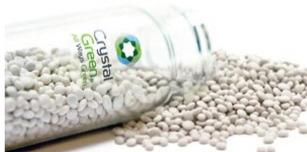
Figure 9.1 Crystal Green™ struvite from sewage sludge
