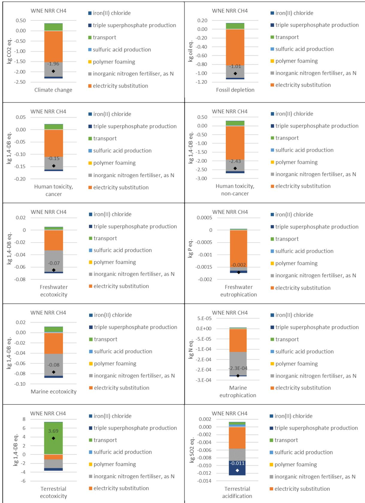
Fig. 2.28: LCIA – Waterleau New Energy (WNE) with NRR per  $m^3 CH_4$
