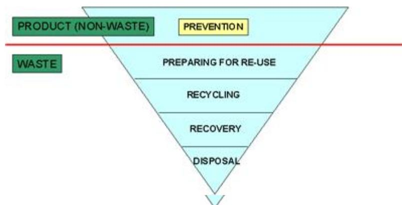
**Fig. 3 Waste hierarchy as stipulated in the Waste Framework Directive (Source [7])**
