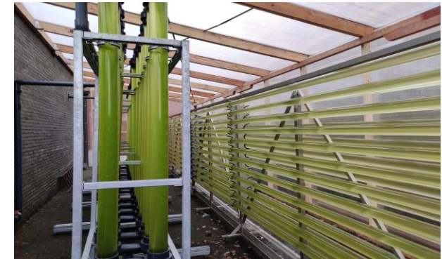
2T photobioreactor Consortium of Chlorella sp. and Desmodesmus sp. 5% of filtered digestate (origin: plant and food waste)
