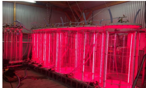
2T photobioreactor Auriantochitrium mangrovei 80% of centrifuged digestate (origin: pig manure)
