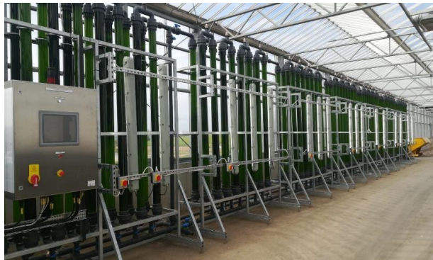
5T photobioreactor Chlorella sp. and Scenedesmus sp. 2.5% of micro-filtered digestate (origin: kitchen waste)
