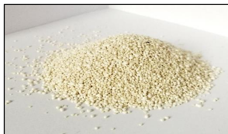
Figure 2 Struvite produced from the processing of wastewater from potato processing company using the NuReSys ® technology.
