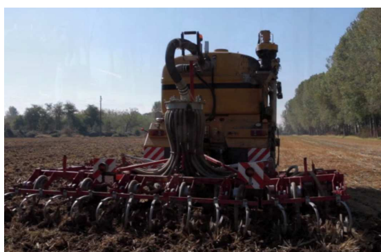
Figure 2. Digestate injection application on fields.
