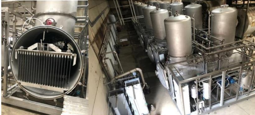
*Figure 2.2 The vacuum evaporator installed at the demonstration plant AM-Power (2019).*
