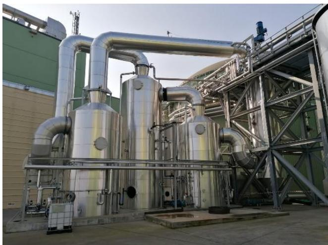
Figure 3.2 Photo of the N absorber installed at the demonstration plant *Acqua&Sole* (2020).
