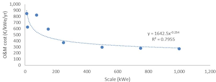
**Figure 4.** *Operating and maintenance cost pocket digester + CHP*
