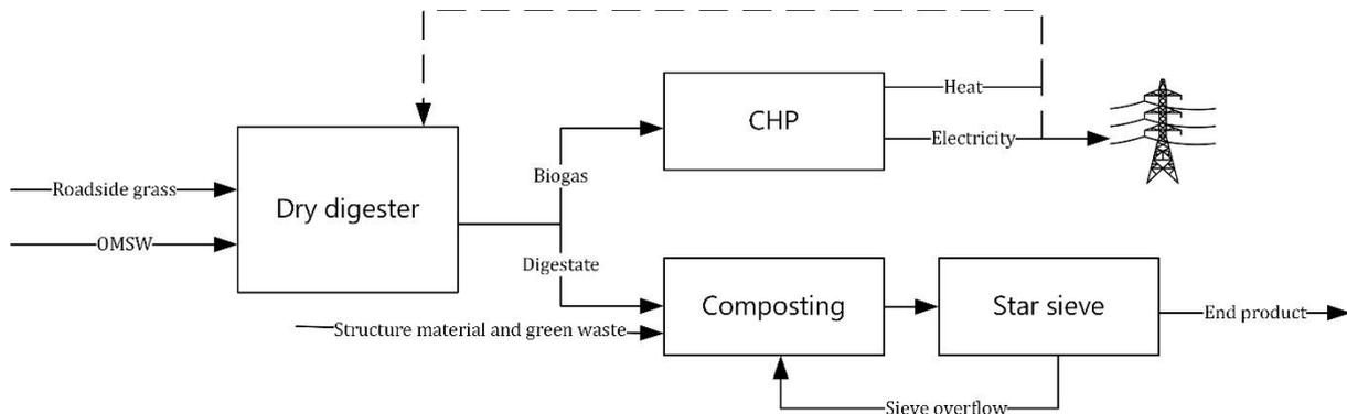
**Figure 6.** *Process flow diagram - reference case 2*
