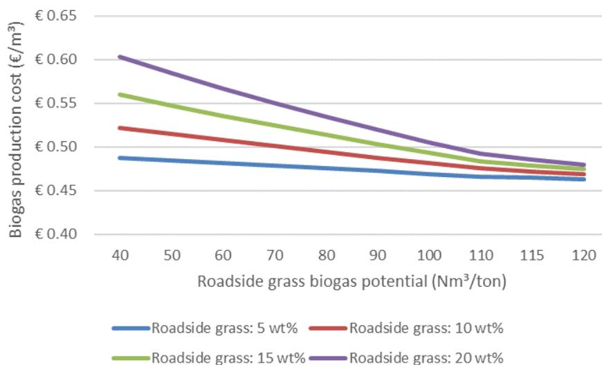
**Figure 10.** *Impact roadside grass amount and biogas yield on biogas production cost – base case*
