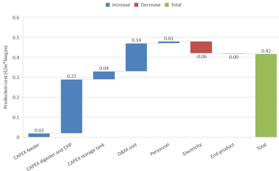
**Figure 12.** Cost breakdown per  $m^3$  of biogas produced – reference case 1
