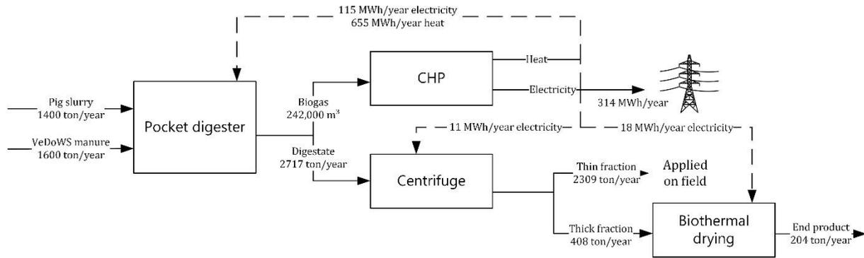
**Figure 11.** *Mass and energy balance – reference case 1*
