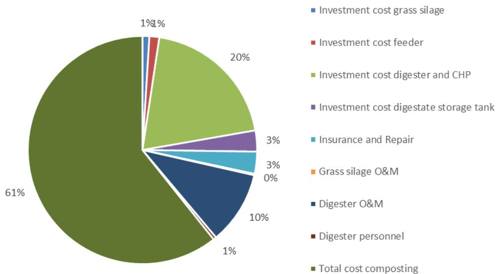
**Figure 8.** Cost breakdown – base case
