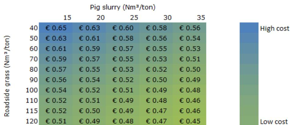
**Figure 9.** Impact biogas yield on biogas production cost – base case
