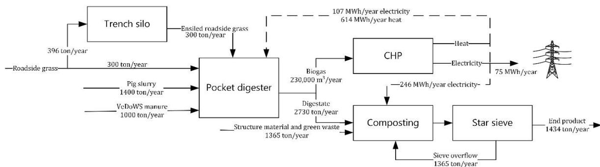
**Figure 7.** *Mass and energy balance – base case*
