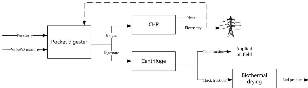
**Figure 5.** Process flow diagram - reference case 1
