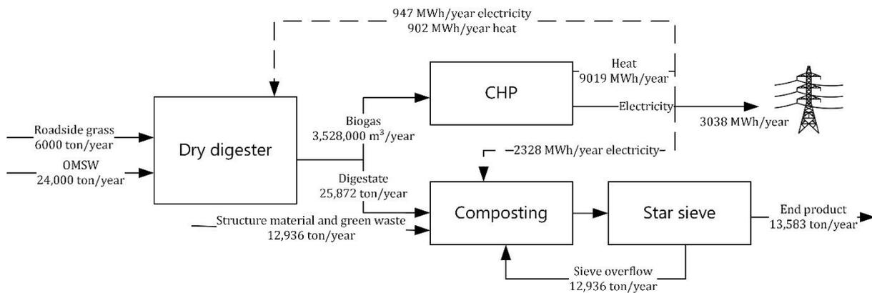
**Figure 13.** Mass and energy balance – reference case 2
