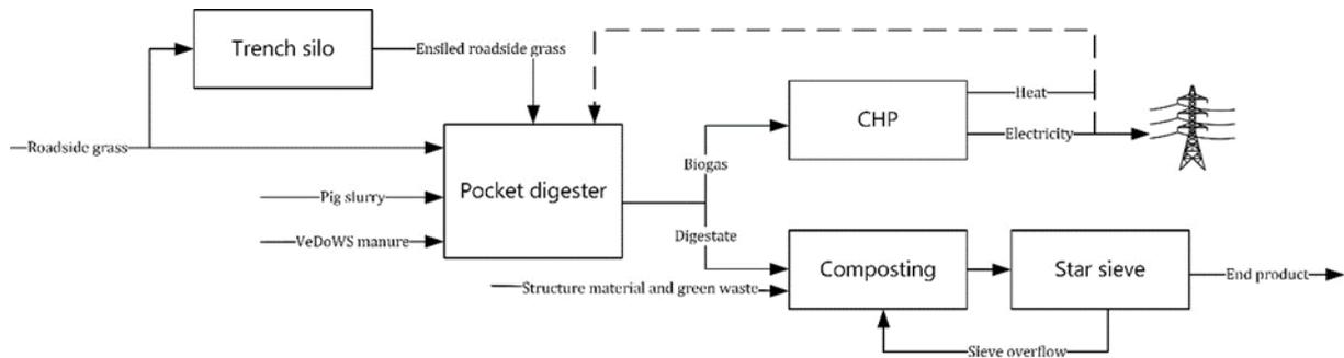
**Figure 2.** Process flow diagram - base case
