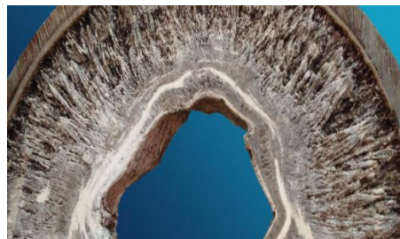
Figure 3: Struvite incrustations in pipes
