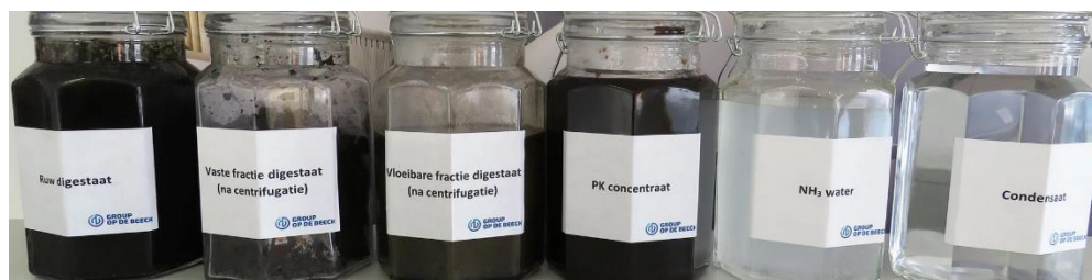
Figure 4: Raw digestate, solid fraction of digestate, liquid fraction of digestate, PK-rich concentrate, \text{NH}_3 water and condensate produced by Group op de Beeck
