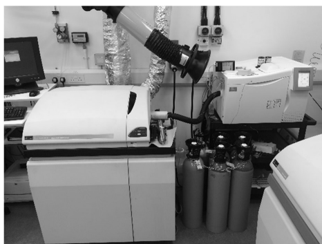
Figure 3: GC-ICP-MS setup for the measurement of total silicon in gaseous reference samples
