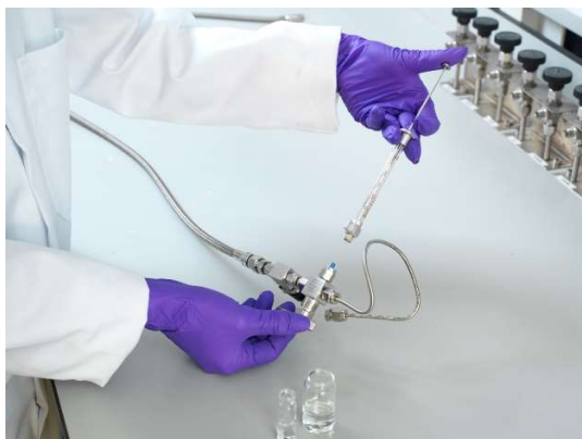
Figure 1: Injection of pure siloxane into transfer vessel prior to high-accuracy weighing
