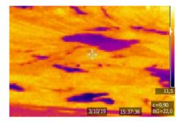
3/10/19: end of batch 1, no isolation panels installed nor heating system. The purple zones are the result of small water puddles on the HDPE surface.
