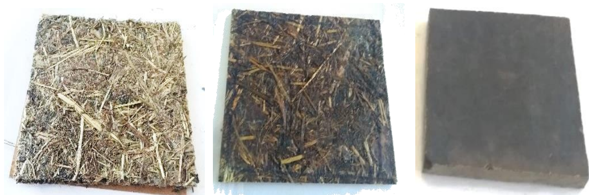
Figure 12: Grass clipping fibreboard prototypes made with varying amounts of biobased binder
