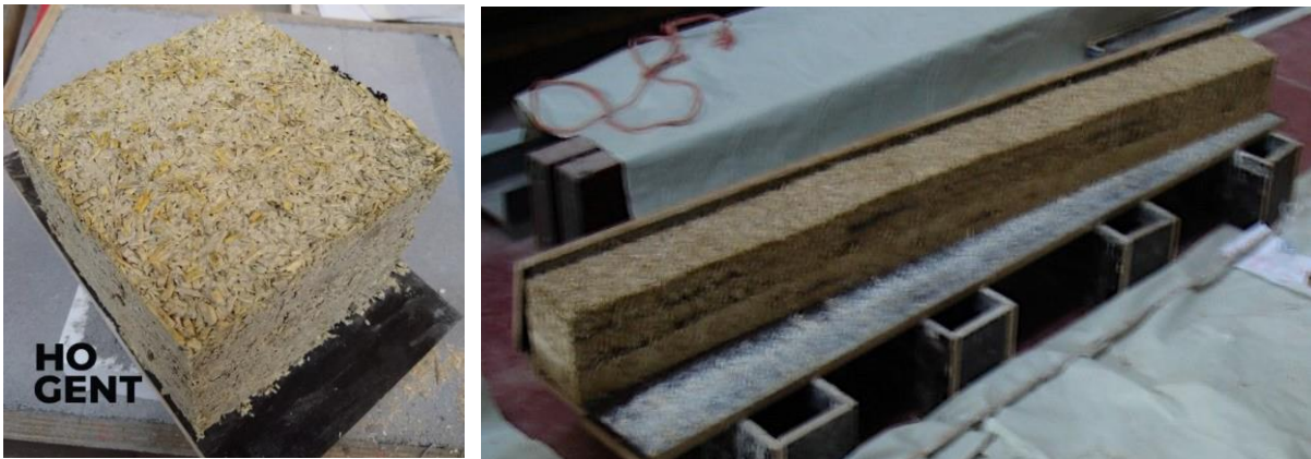
Figure 13: “Grass-crete” beam and block made of dried grass clippings and lime. The beam was reinforced with “lianas” of hop stems. The block contained hemp shives also.
