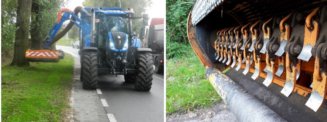
Figure 1: (left) Flail mower mowing of roadside in the commune of Harelbeke with (right) an adapted mowing head (Vandaele).
