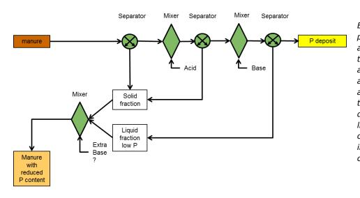
Example of scheme showing how pig slurry is separated into a liquid and a solid fraction. Acid is added to the liquid phase, that is mixed and separated again into a solid and a liquid fraction. Solid fractions are combined, and base is added to the liquid fraction from which a P deposit is separated for reuse. A liquid fraction remains that can be combined with the solid fractions into manure with a lowered P content.
