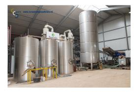
Greendal vergisting biogas plant is based on a chicken farm, with the idea to use a high share of chicken litter as substrate (> 50%). Due to the high nitrogen loading such a high percentage of chicken litter in the substrate has not been used in any plant before.
