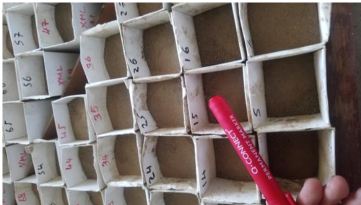
Figure 9 Dried 2 mm sieved soil samples in cardboard box for nutrient and metal analysis.
