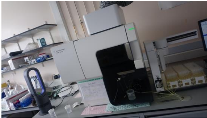
Figure 10 ICP-OES spectrometer facility to analyse soil samples for nutrients and metals.
