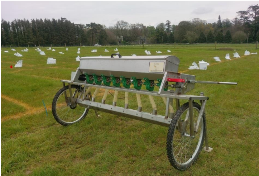
Figure 6: 2 m wide barrow fertilizer spreader for applying mineral fertilizer to relevant plots at pre-calibrated rates.
