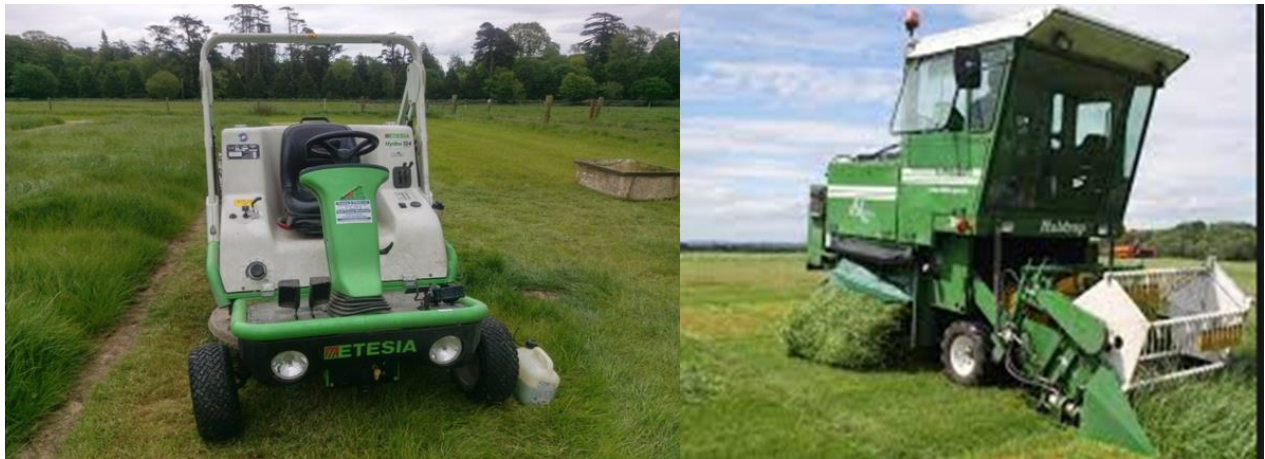
Figure 12 Etesia trial plot mower with a 1.24 m cutting width and 5cm cutting height (left) and a Haldrup combine harvester (right).
