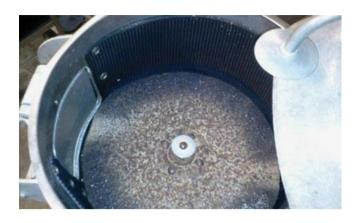
**Figure 7 (left)** Abrasion peeler for potatoes and sweet potatoes. **(right)** Rotating cylinder with an abrasive surface along the inner wall to remove the skins as the cylinder rotates.
