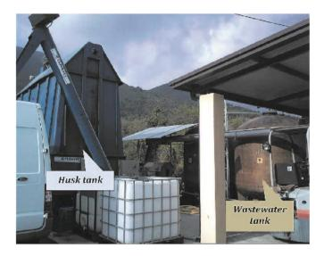
Figure 19 Tanks for the collection of olive processing by-products at the end of production system.
