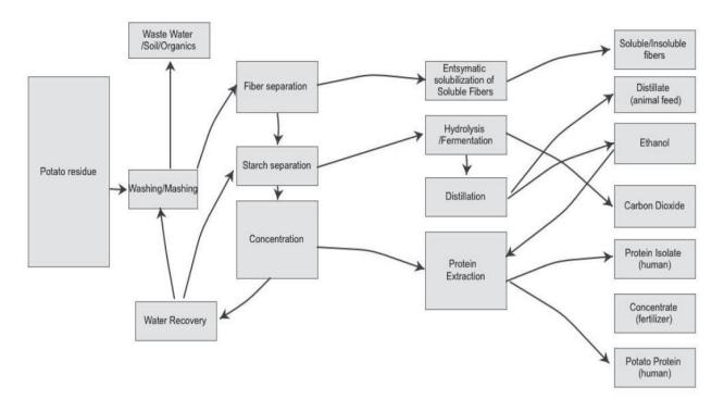
Figure 18 Flow chart of value added products from potato residue feedstock [267].
