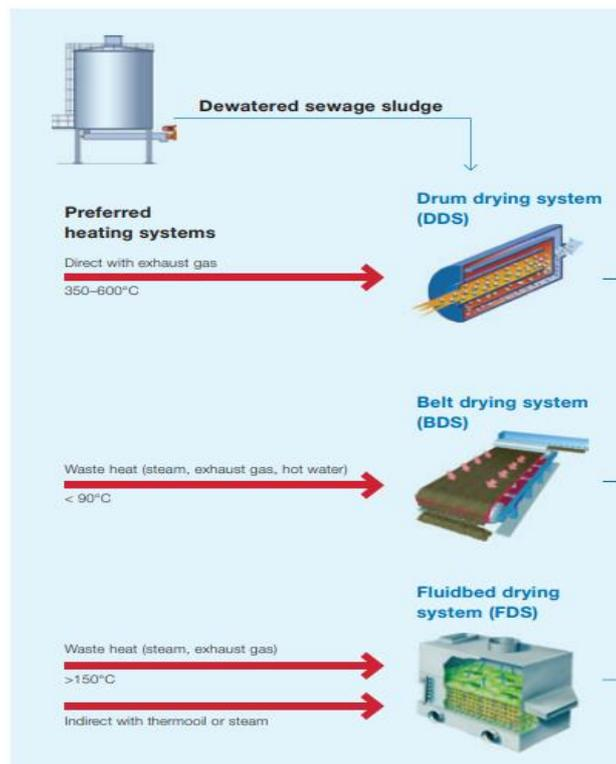
**Figure 7.** Three types of drying systems in use by Andritz Dryers based on temperatures and heat source (Andritz, 2012).
