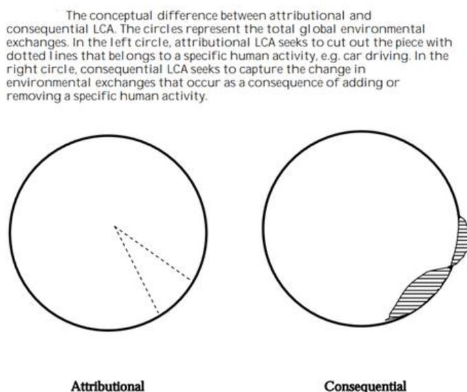
**Figure 2.** *Conceptual difference between aLCA and cLCA (Ekvall et al., 2016)*
