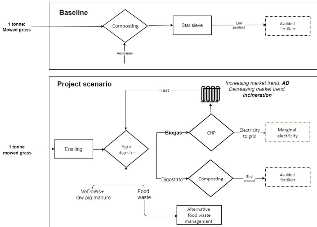
**Figure 3.** System boundaries for LCA. Dotted lines indicate avoided processes
