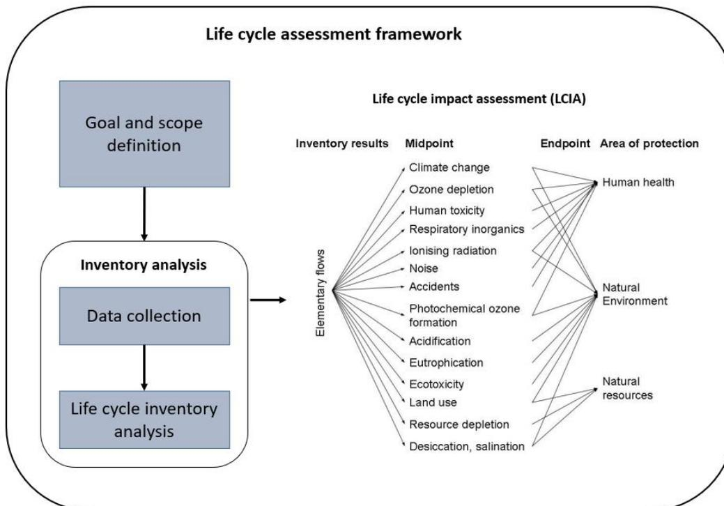
**Figure 1.** Phases of an LCA (Adapted from ISO 14040)
