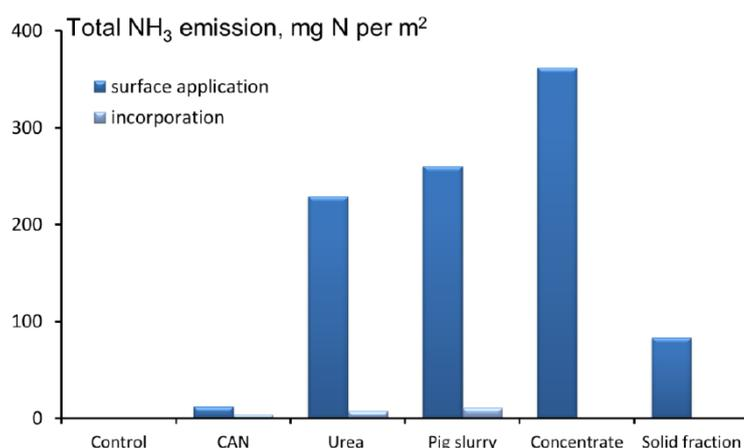
Total  $\text{NH}_3$  emission in 28 days from calcium ammonium nitrate (CAN), urea, untreated pig slurry, mineral concentrate and the solid fraction from separated slurry (averages of four farms) applied to arable sandy soil.
